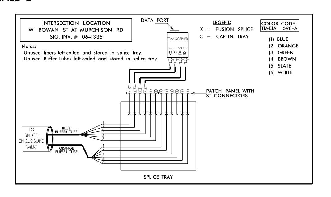
INCLUDE ON THE COVER OF EACH SPLICE TRAY THE FOLLOWING: REFERENCE SECTION 1731 "FIBER OPTIC SPLICE ENCLOSURE"
