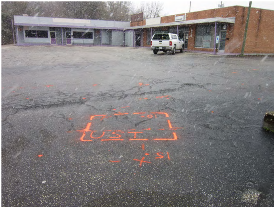
Parcel 020 (Unassigned AKA P&S Enterprises Property), looking north. Photo shows approximate marked location of Probable UST No. 1 near the southwest end of the canopy on Parcel 020.
