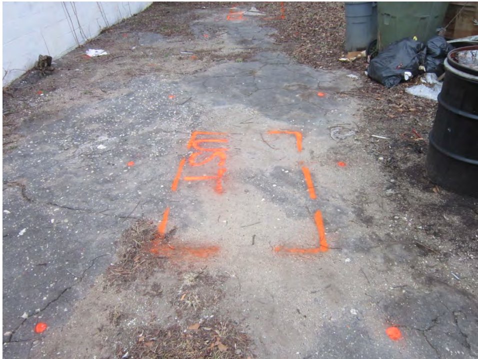
Parcel 007 (Edmund George Property), looking north. Photo shows approximate marked location of Probable UST No. 2 near the southeast corner of the building on Parcel 007
