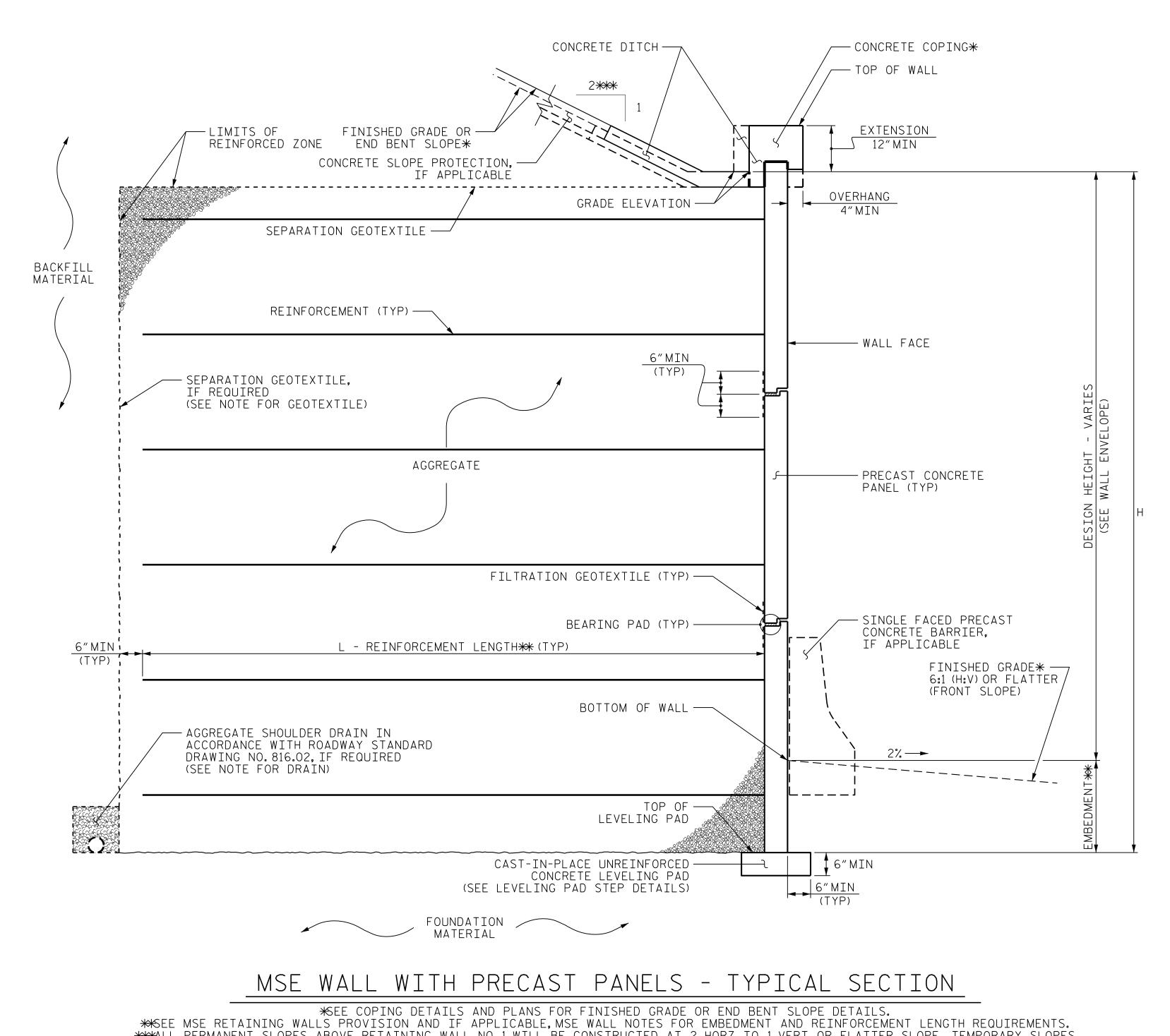
\*\*\*ALL PERMANENT SLOPES ABOVE RETAINING WALL NO.1 WILL BE CONSTRUCTED AT 2 HORZ. TO 1 VERT. OR FLATTER SLOPE. TEMPORARY SLOPES DURING CONSTRUCTION WILL BE CONSTRUCTED AT 1.5 HORZ. TO 1 VERT. OR FLATTER SLOPE.
