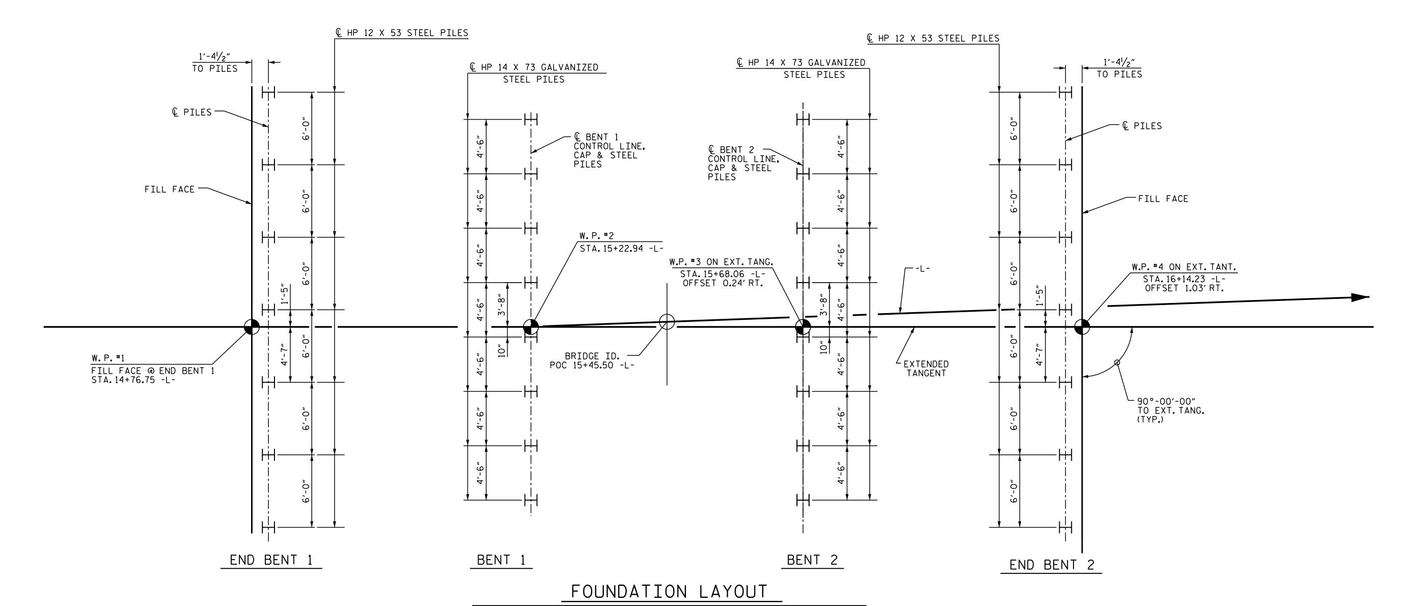
DIMENSIONS LOCATING PILES ARE SHOWN TO THE PILE CENTERLINE.
