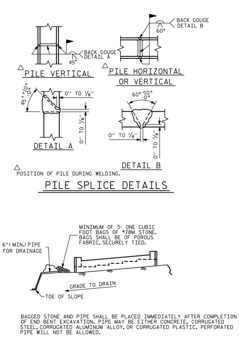
BAGGED STONE SHALL REMAIN IN PLACE UNTIL THE ENGINEER DIRECTS THAT IT BE REMOVED. THE CONTRACTOR SHALL REMOVE AND DISPOSE OF SILT ACCUMULATIONS AT BAGGED STONE WHEN SO DIRECTED BY THE ENGINEER. BAGS SHALL BE REMOVED AND REPLACED WHENEVER THE ENGINEER DETER-MINES THAT THEY HAVE DETERIORATED AND LOST THEIR EFFECTIVENESS.
