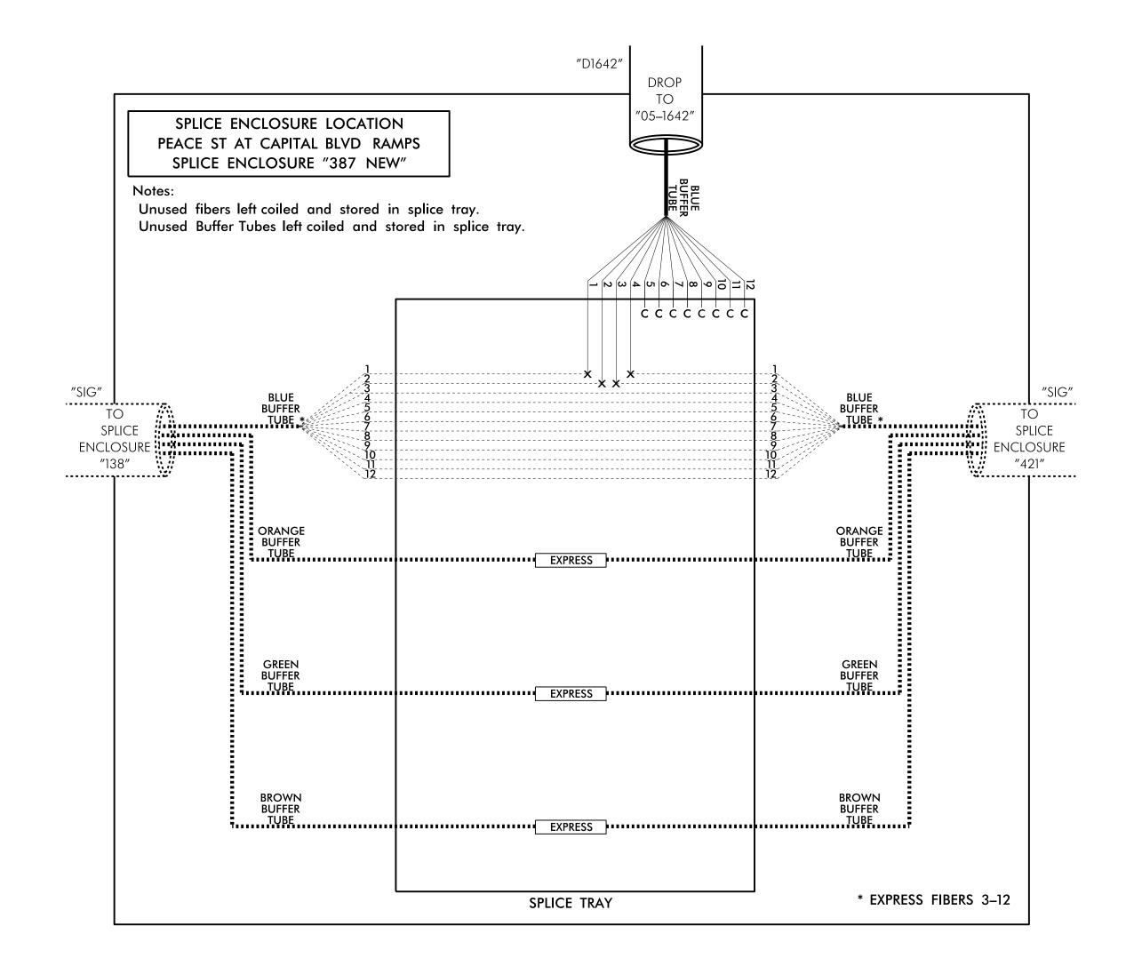
CONTRACTOR TO RECORD EXISTING SPLICE ARRANGEMENT FOR COMPARISON TO THE SUPPLIED SPLICE PLANS. IF DISCREPANCIES EXIST, CONTACT THE ENGINEER TO DETERMINE HOW TO PROCEED WITH RESPLICING.
