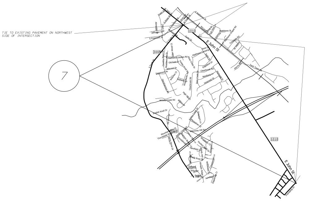
IN THIS SECTION ONLY MILL AND PATCH IN VARIOUS AREAS AS DETERMINED BY THE ENGINEER. PATCHES ARE TO BE CAPPED WITH SURFACE COURSE IN A MANNER TO ACCEPT PERMANENT TRAFFIC.
