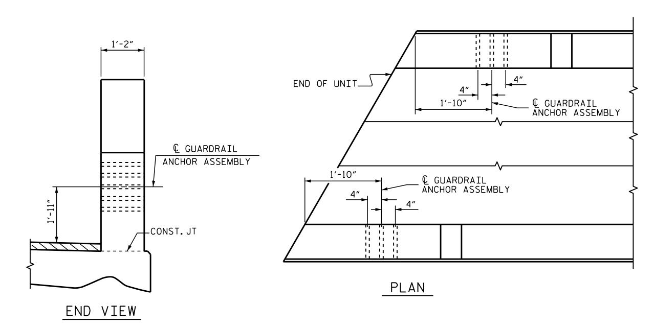
LOCATION OF GUARDRAIL ANCHOR AT END POST ASSEMBLED BY : M. POOLE DATE : 01-16 CHECKED BY : M. G. CHEEK DATE : 2-12-16 DRAWN BY: MAA 5/10 CHECKED BY: GM 5/10 REV. 12/5/11 MAA/GM
