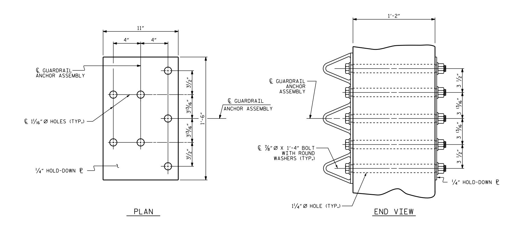
GUARDRAIL ANCHOR ASSEMBLY DETAILS
