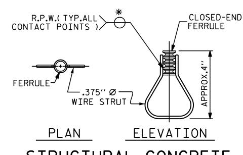
STRUCTURAL CONCRETE \* EACH WELDED ATTACHMENT OF WIRE TO
