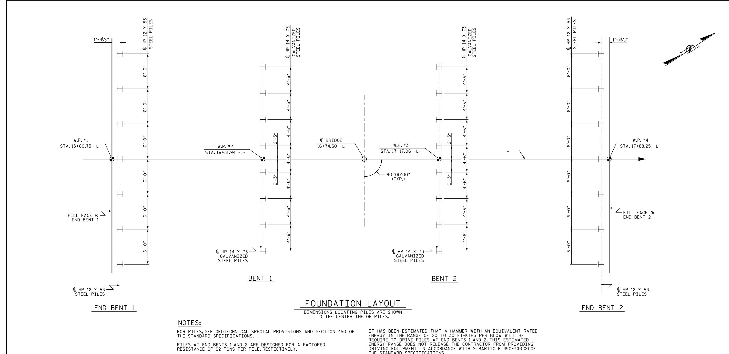
DRIVE PILES AT END BENTS 1 AND 2 TO A REQUIRED DRIVING RESISTANCE OF 155 TONS PER PILE, RESPECTIVELY.
