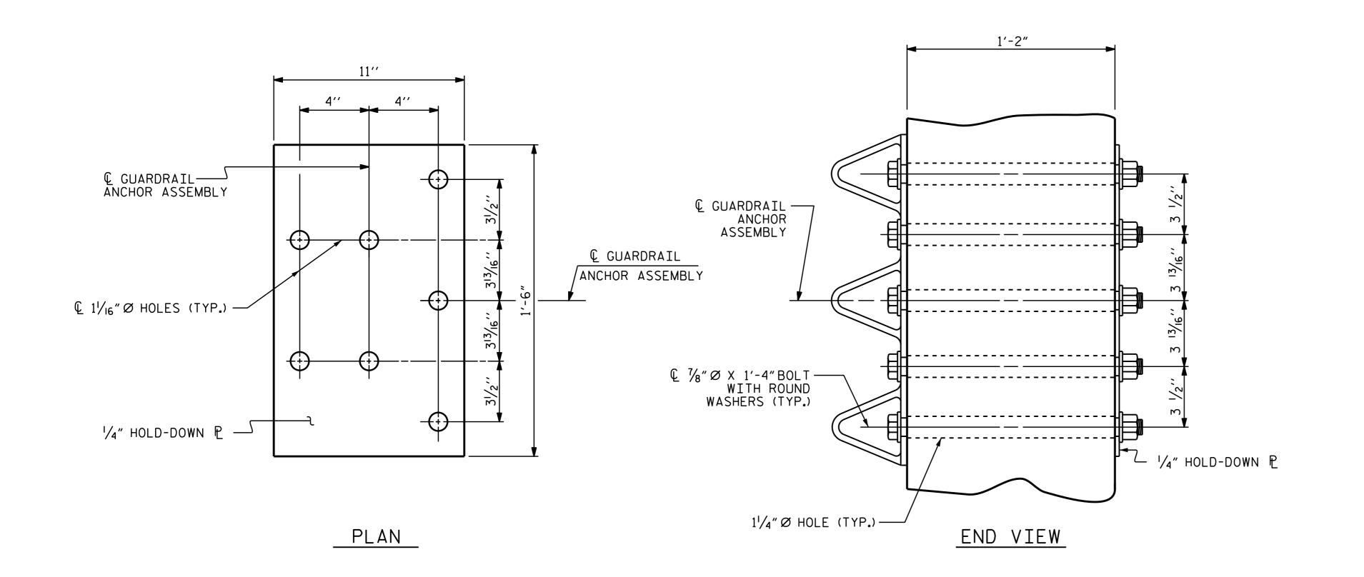
GUARDRAIL ANCHOR ASSEMBLY DETAILS
