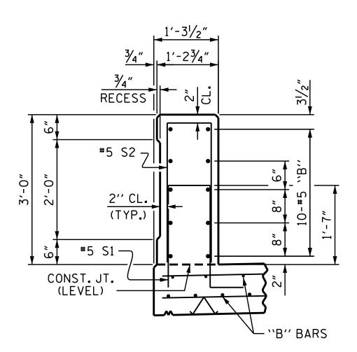
SECTION THROUGH PARAPET
