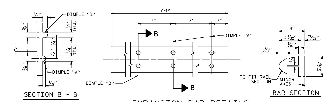
1/2" Ø [13 THREAD] HOLE FOR 1/2" Ø X 1" STAINLESS STEEL HEX HEAD CAP SCREW & 1/16" O.D., 17/32" I.D.,
