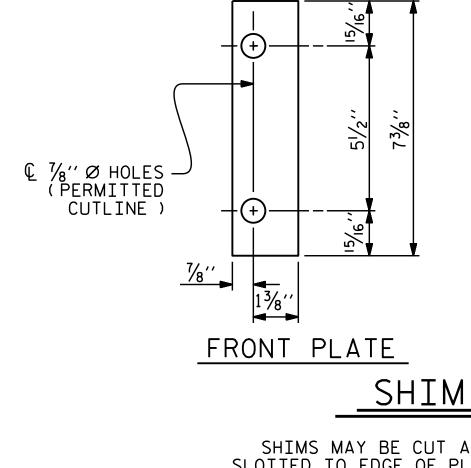
SHIM DETAILS SHIMS MAY BE CUT ALONG PERMITTED CUTLINE OR SLOTTED TO EDGE OF PLATE TO FACILITATE PLACEMENT.
