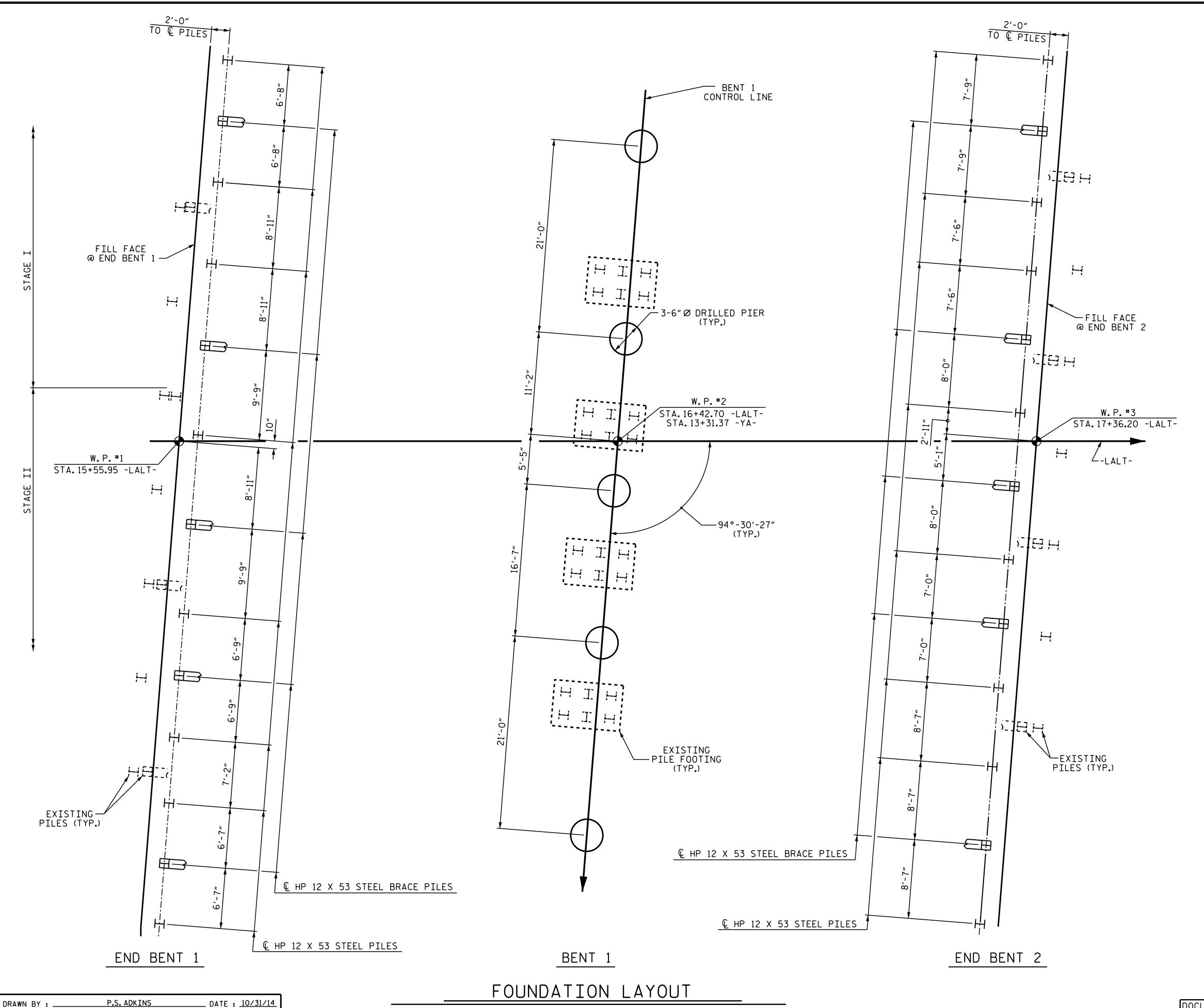
DIMENSIONS LOCATING PILES ARE SHOWN TO THE CENTERLINE OF PILES. DIMENSIONS FOR DRILLED PIERS ARE SHOWN TO THE CENTERLINE OF DRILLED PIERS.
