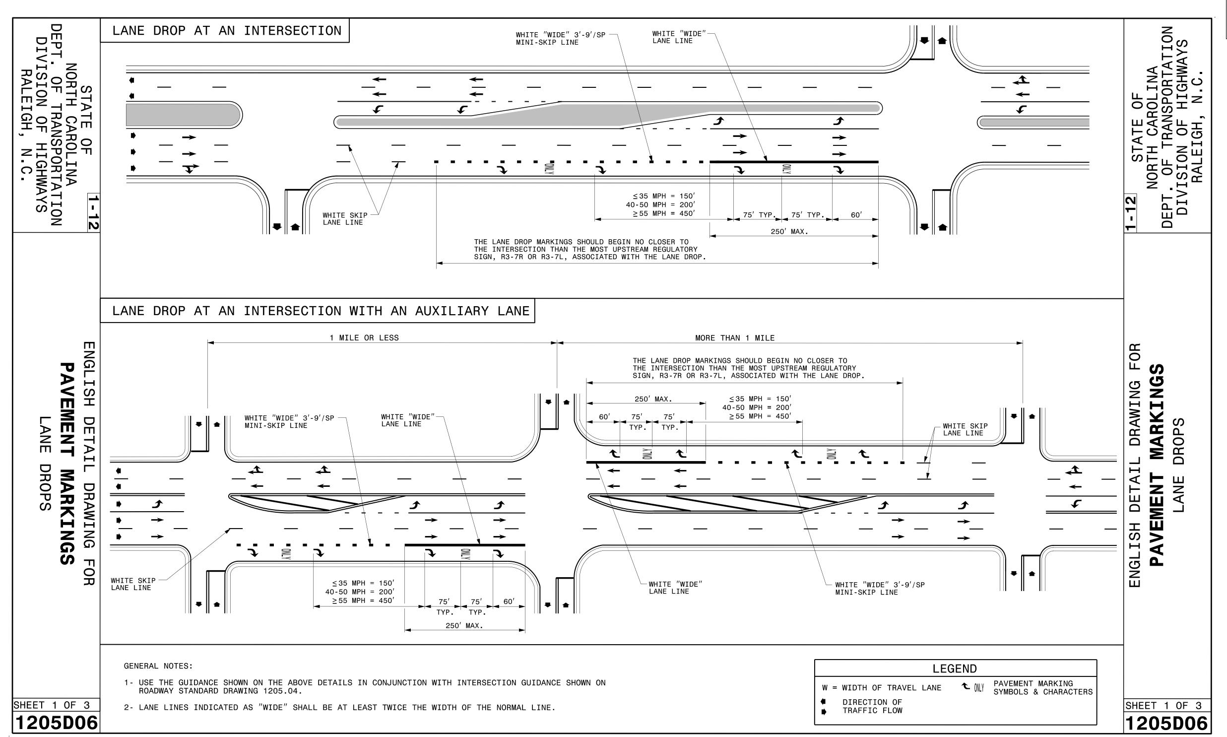
REVISED PAVEMENT MARKING ROADWAY STANDARD DRAWING
