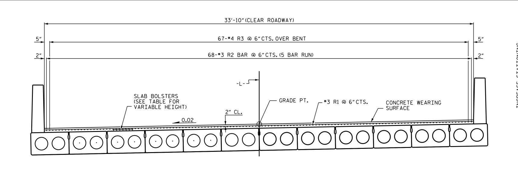
REINFORCING FOR CONCRETE WEARING SURFACE
