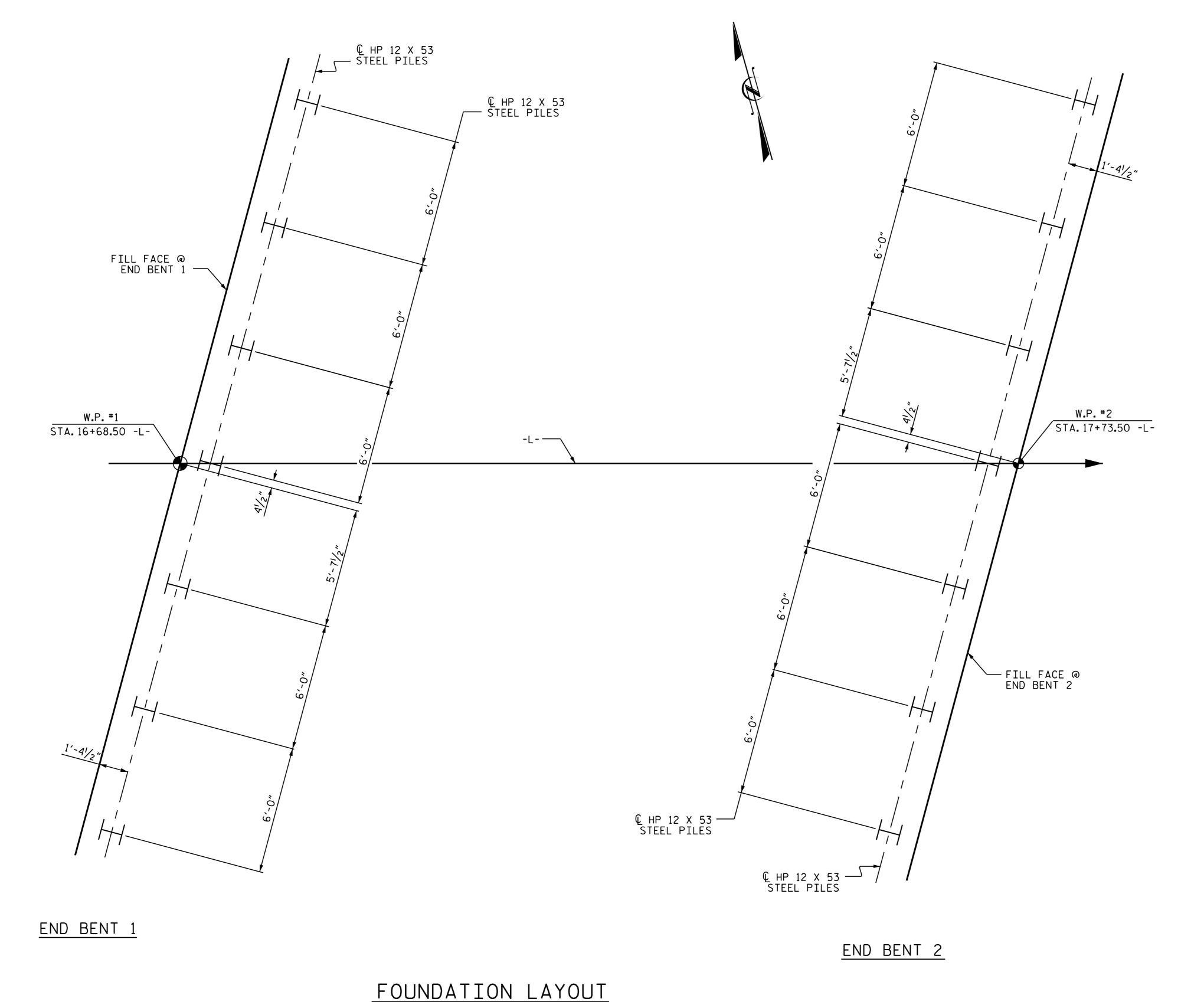
DIMENSIONS LOCATING PILES ARE SHOWN TO THE CENTERLINE OF PILES.
