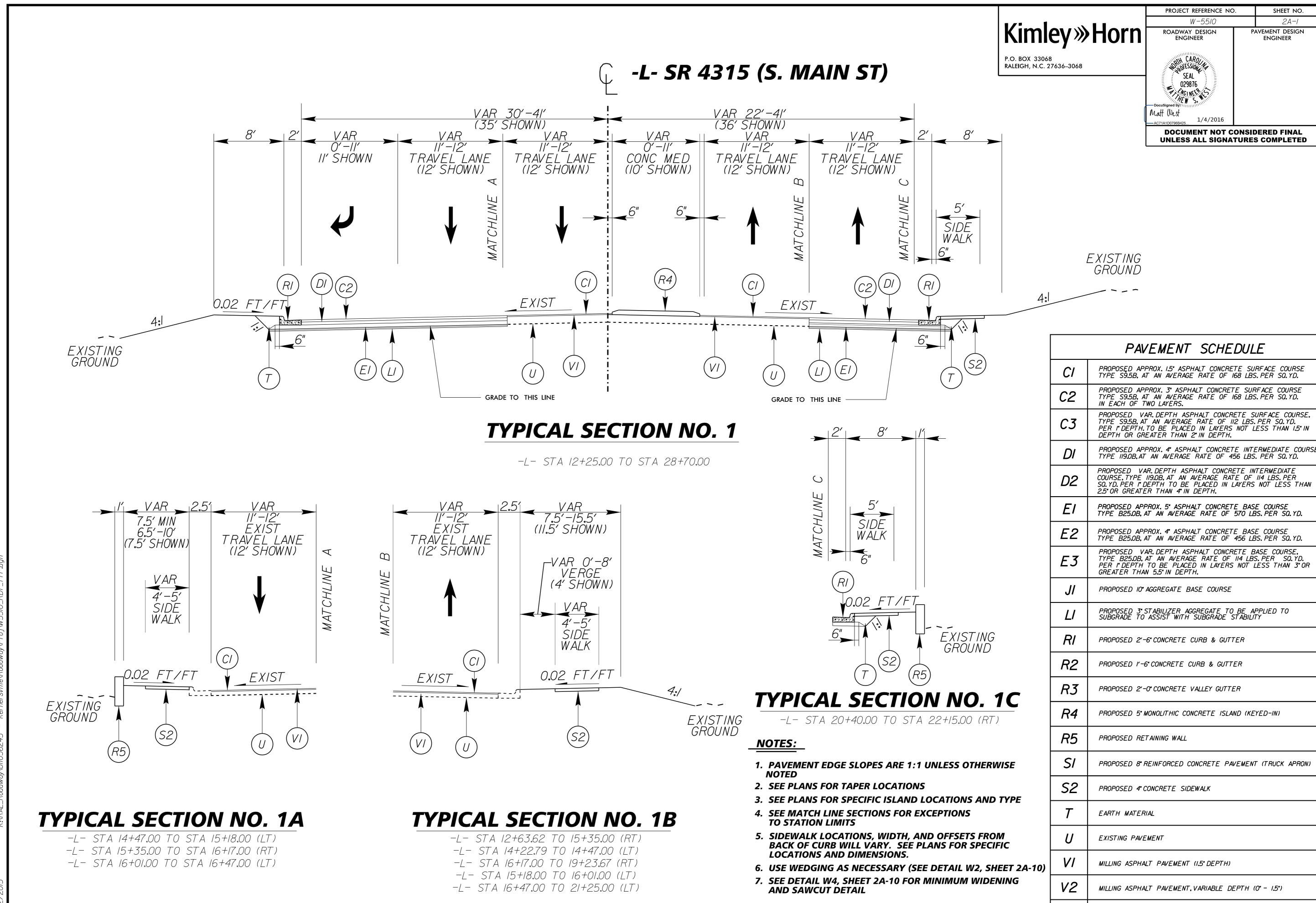
VARIABLE DEPTH ASPHALT PAVEMENT (SEE DETAIL W2,SHEET 2A-10)
