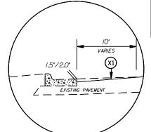
DETAIL FOR PROFILE MILLING (0" TO 1.5") DETAIL FOR PROFILE MILLING (0" TO 2.0")
