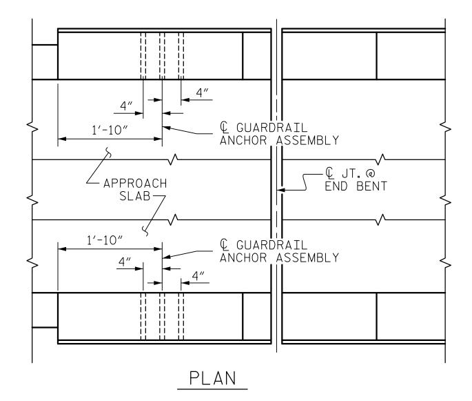
LOCATION OF GUARDRAIL ANCHOR AT END POST
