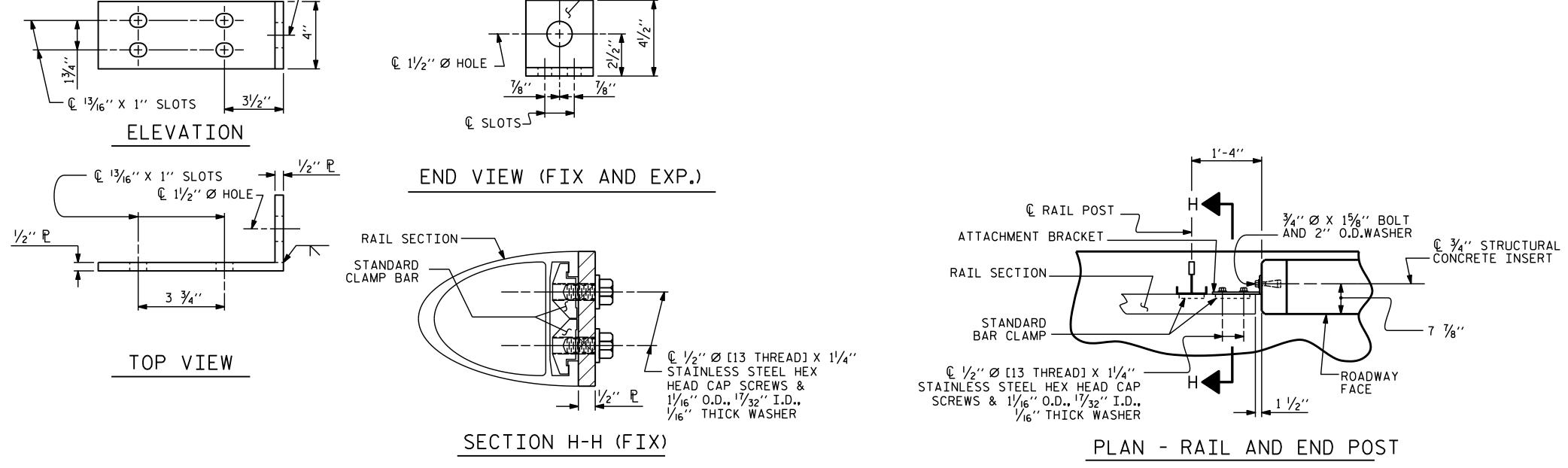
DETAILS FOR ATTACHING METAL RAIL TO END POST
