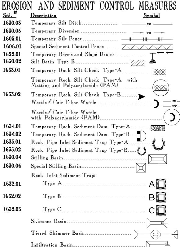
THIS PROJECT CONTAINS EROSION CONTROL PLANS FOR CLEARING AND GRUBBING PHASE OF CONSTRUCTION.
