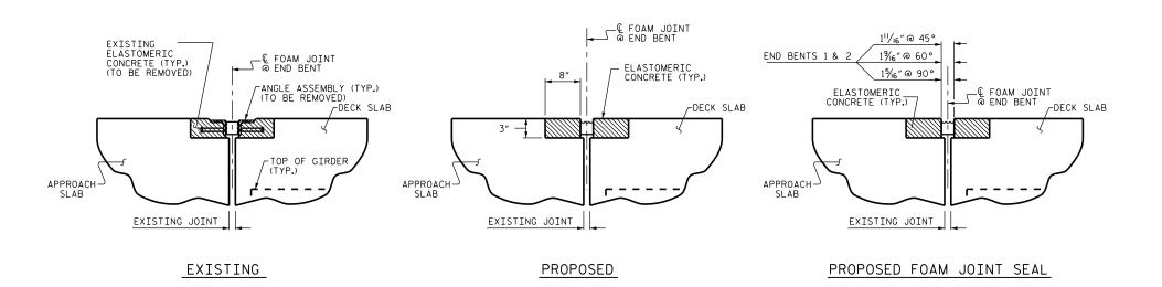
JOINT SEAL DETAILS AT END BENT
