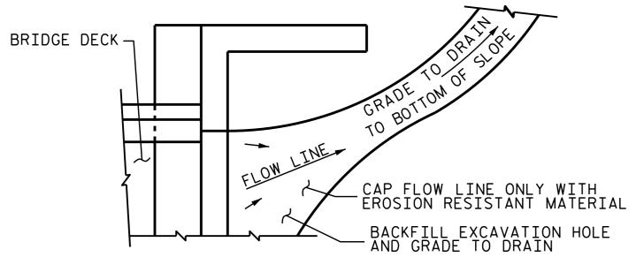
TE: IF THE APPROACH SLAB IS NOT CONSTRUCTED IMMEDIATELY AFTER THE BACKFILLING OF THE END BENT EXCAVATION, GRADE TO DRAIN TO THE BOTTOM OF THE SLOPE AND PROVIDE EROSION RESISTANT MATERIAL, SUCH AS FIBERGLASS ROVING OR AS DIRECTED BY THE ENGINEER TO PREVENT SOIL EROSION AND TO PROTECT THE AREA ADJACENT TO THE STRUCTURE. THE CONTRACTOR WILL BE REQUIRED TO REMOVE THESE MATERIALS PRIOR TO CONSTRUCTION OF THE APPROACH SLAB.
