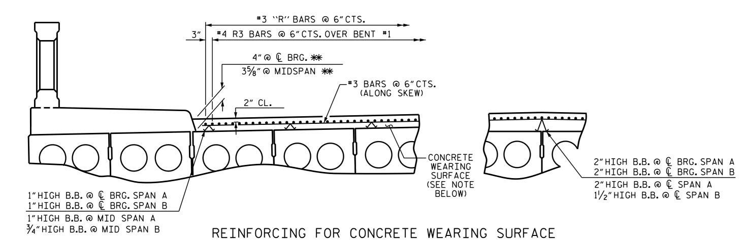
\*\* THICKNESS IS BASED ON PREDICTED FINAL CAMBER & THEORITICAL GRADE LINE ELEVATIONS AND VARIES BETWEEN & BEARING AND MID-SPAN FOR ALL SPANS.
