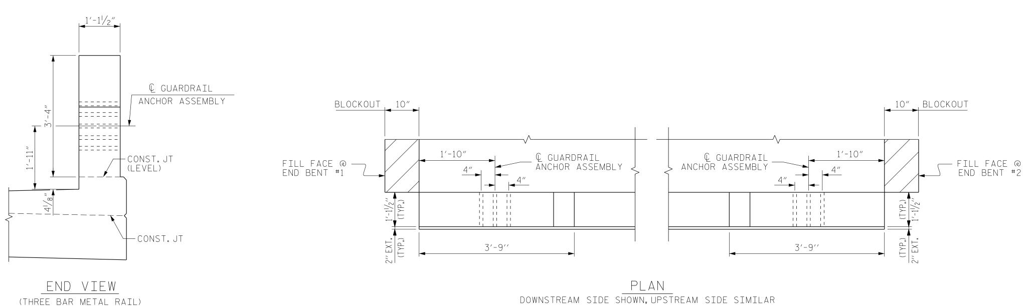
LOCATION OF GUARDRAIL ANCHOR AT END POST
