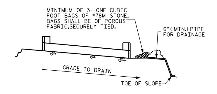
BAGGED STONE AND PIPE SHALL BE PLACED IMMEDIATELY AFTER COMPLETION OF END BENT EXCAVATION. PIPE MAY BE EITHER CONCRETE, CORRUGATED STEEL, CORRUGATED ALUMINUM ALLOY, OR CORRUGATED PLASTIC. PERFORATED PIPE WILL NOT BE ALLOWED.
