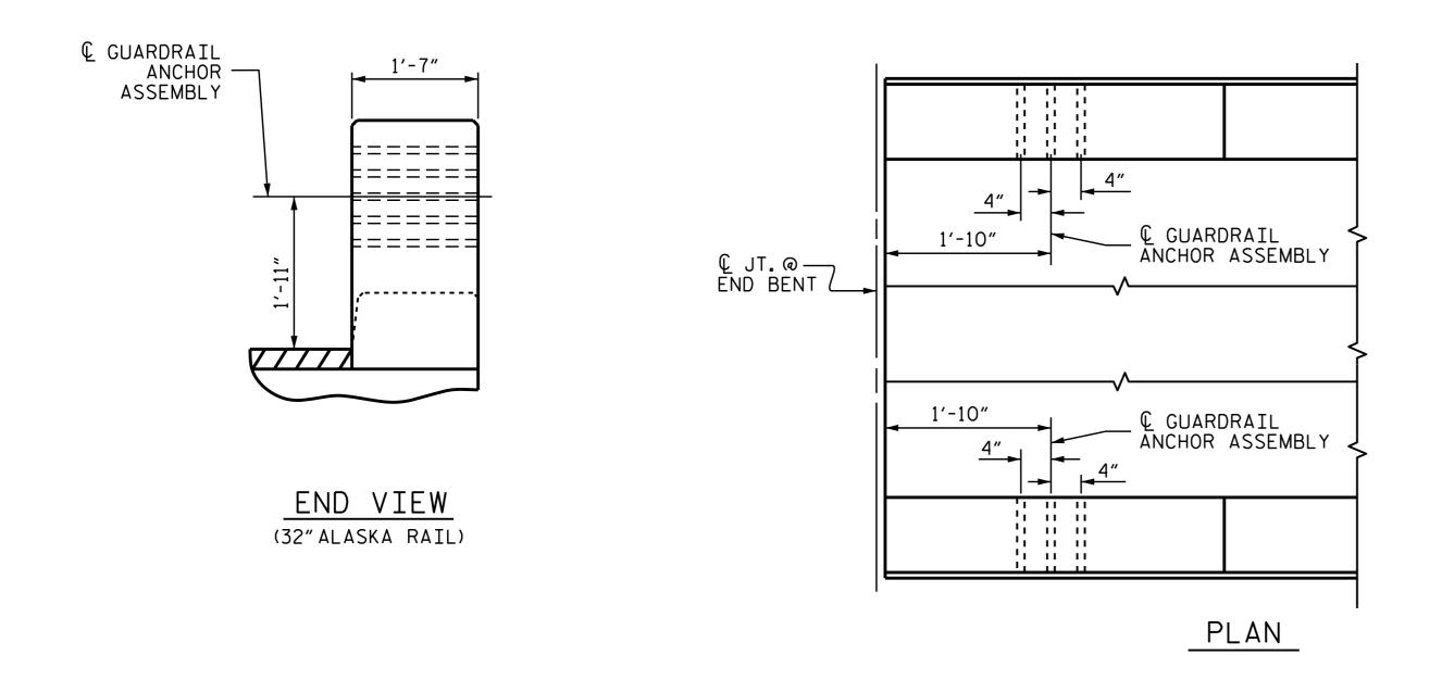
LOCATION OF GUARDRAIL ANCHOR AT END POST
