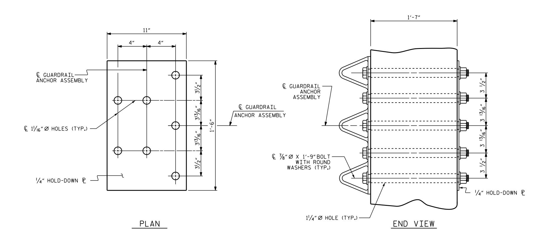
GUARDRAIL ANCHOR ASSEMBLY DETAILS
