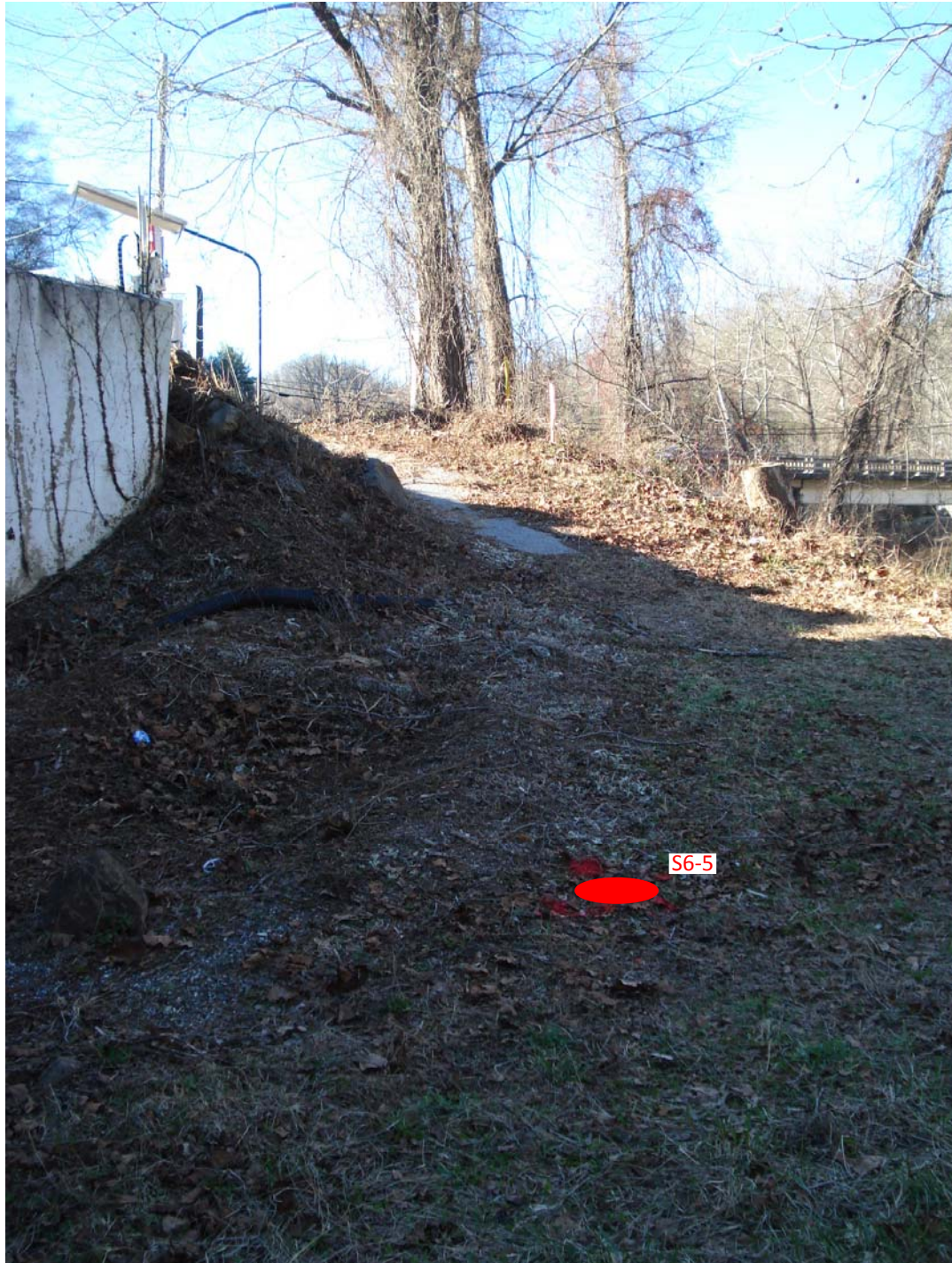
Photograph 3: View looking northwest at soil boring location S6-5. Retaining wall for the 3 known onsite USTs is shown on left, and the Old Cullowhee Road bridge over the Tuckasegee River is shown in background in upper right.
