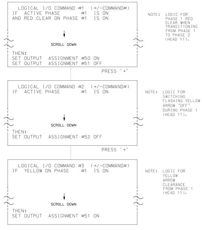
LOGIC I/O PROCESSOR PROGRAMMING COMPLETE
