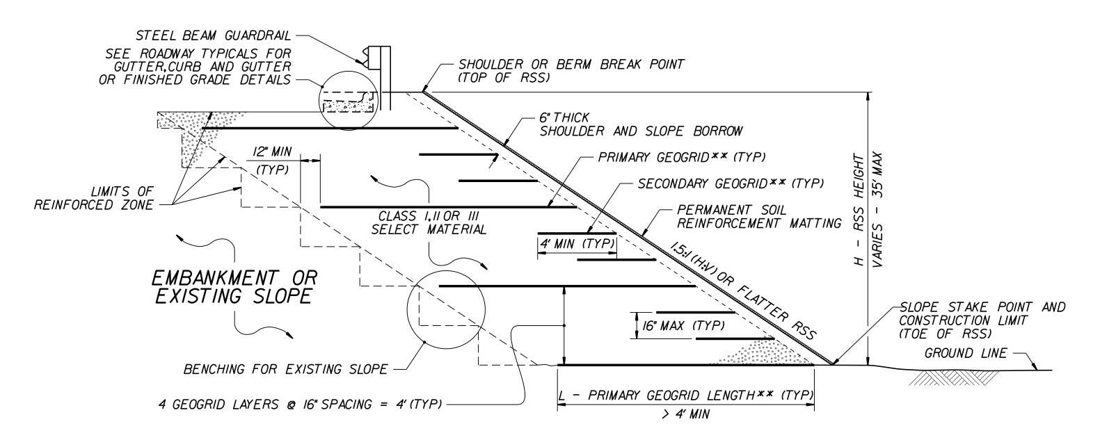
STANDARD RSS WITH SELECT MATERIAL THAT DOES NOT MEET ARTICLE 1019–2 OF THE STANDARD SPECIFICATIONS
