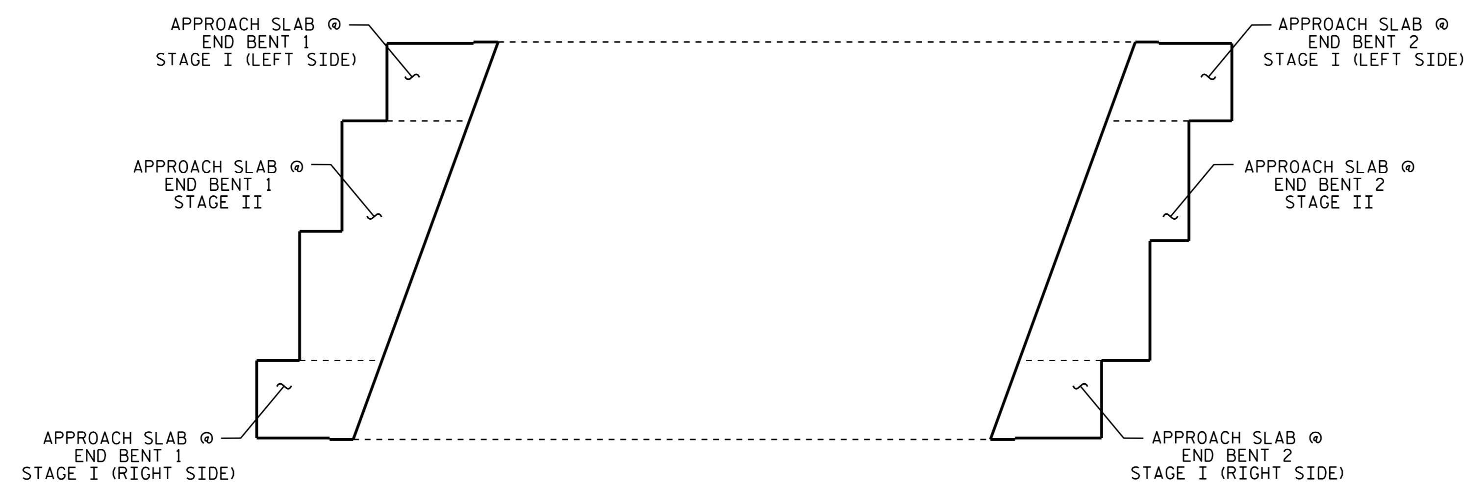
APPROACH SLAB LAYOUT SKETCH
