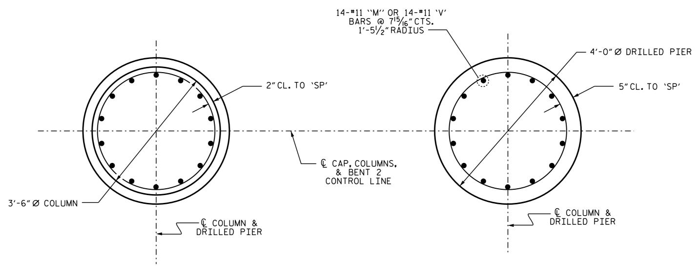
DETAILS OF COLUMNS AND DRILLED PIERS
