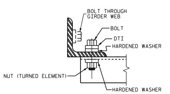
BOLT WITH DTI ASSEMBLY DETAIL
