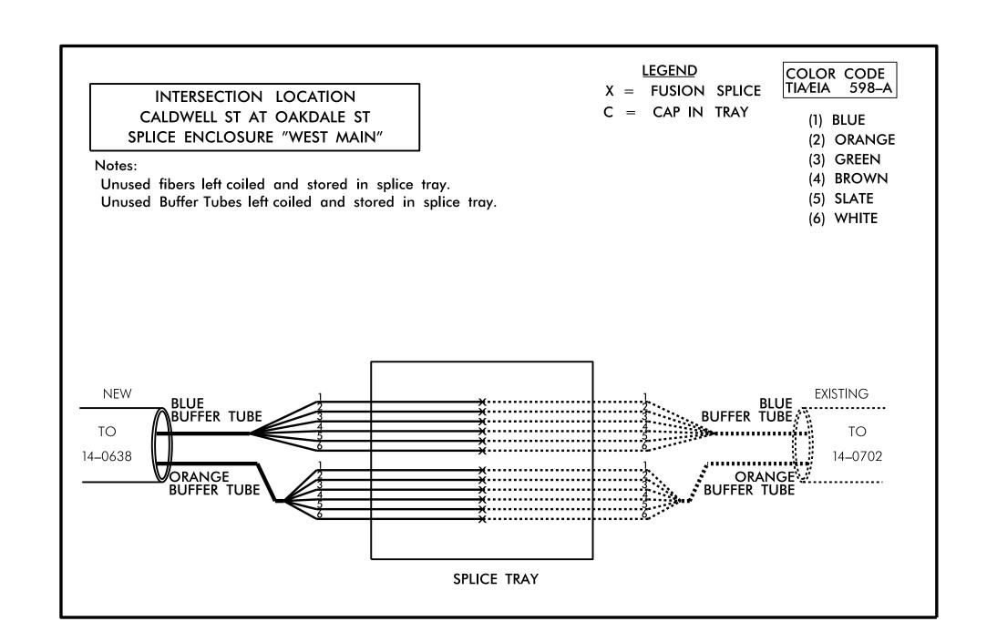
CONTRACTOR TO RECORD EXISTING SPLICE ARRANGEMENT FOR COMPARISON TO THE SUPPLIED SPLICE PLANS. IF DISCREPANCIES EXIST, CONTACT THE ENGINEER TO DETERMINE HOW TO PROCEED WITH RESPLICING.
