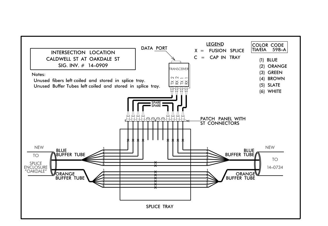
CONTRACTOR TO RECORD EXISTING SPLICE ARRANGEMENT FOR COMPARISON TO THE SUPPLIED SPLICE PLANS. IF DISCREPANCIES EXIST, CONTACT THE ENGINEER TO DETERMINE HOW TO PROCEED WITH RESPLICING.
