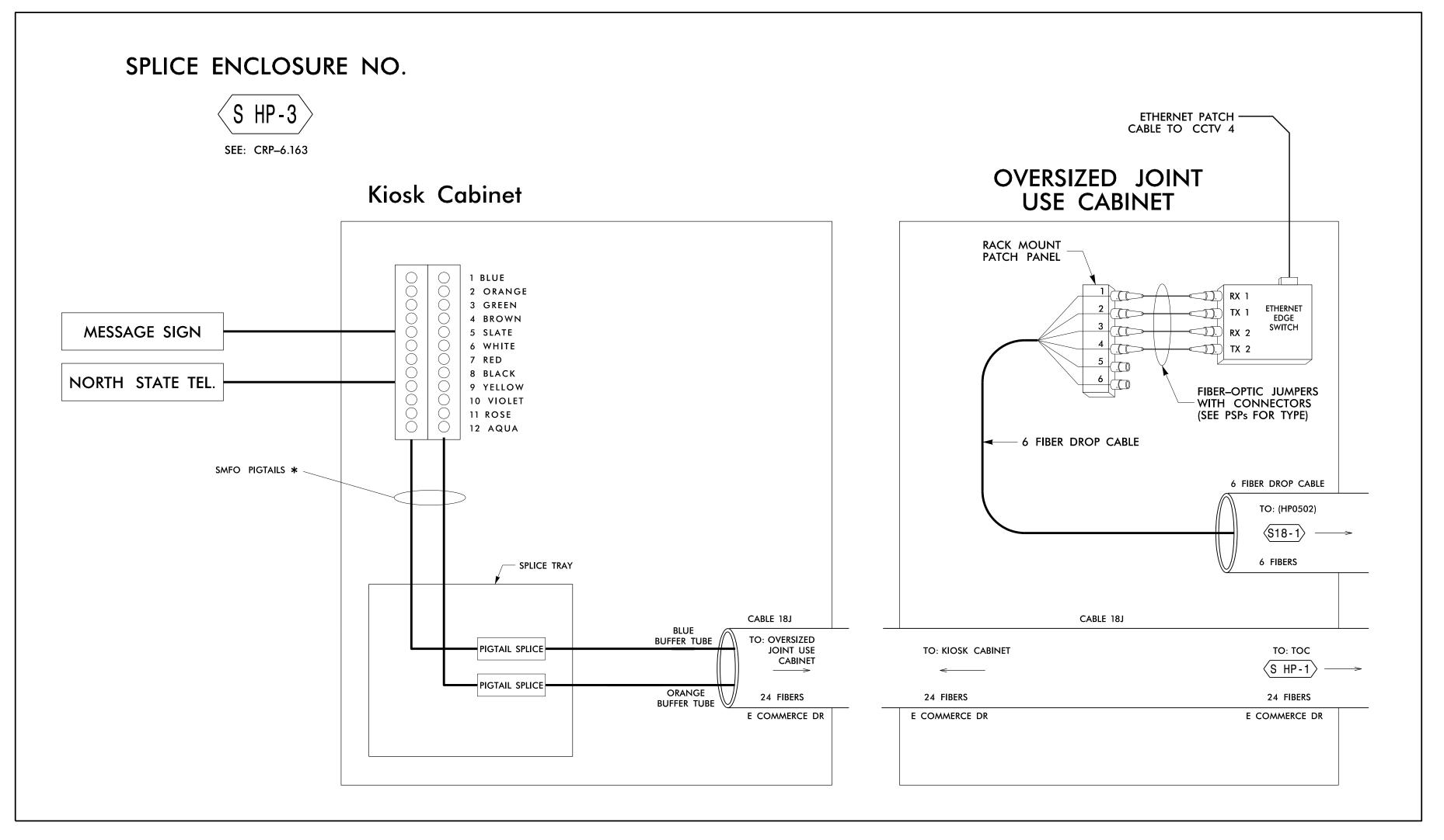
SMFO PIGTAILS TO BE SPLICED TO BUFFER TUBES COLOR TO COLOR.
