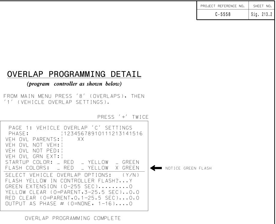
THIS ELECTRICAL DETAIL IS FOR THE SIGNAL DESIGN: HPØ819 DESIGNED: April 2014 SEALED: June 5,2015 REVISED:
