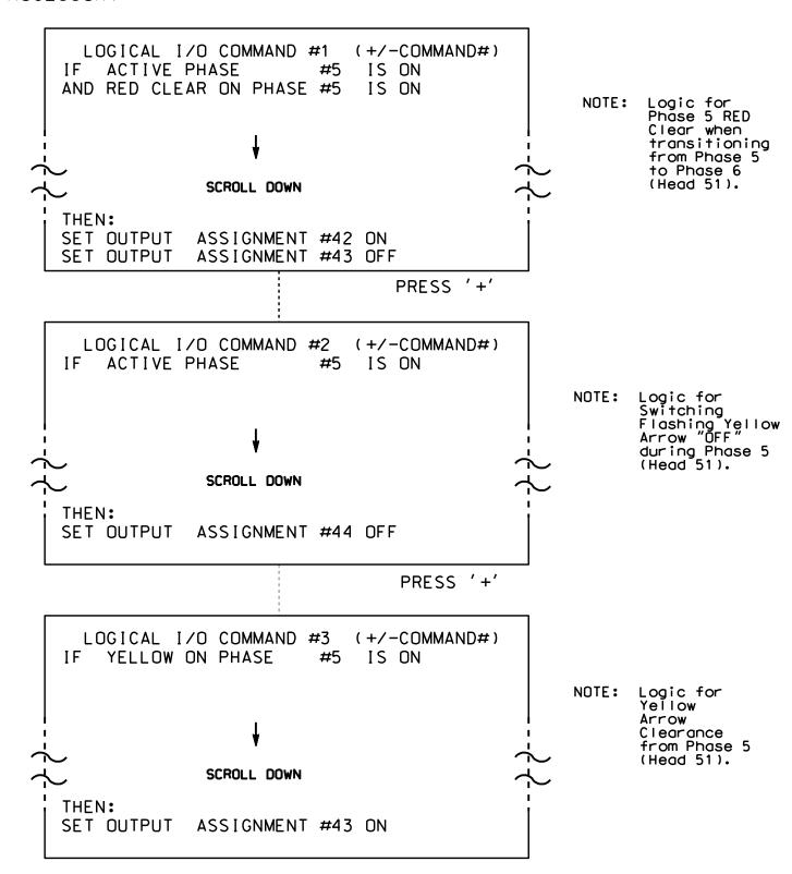
LOGIC I/O PROCESSOR PROGRAMMING COMPLETE
