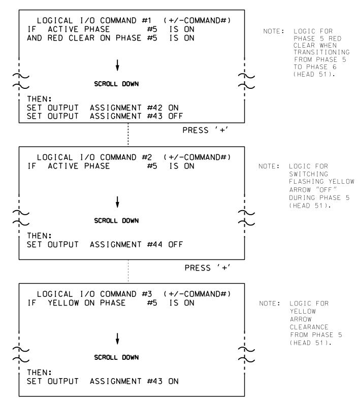
LOGIC I/O PROCESSOR PROGRAMMING COMPLETE
