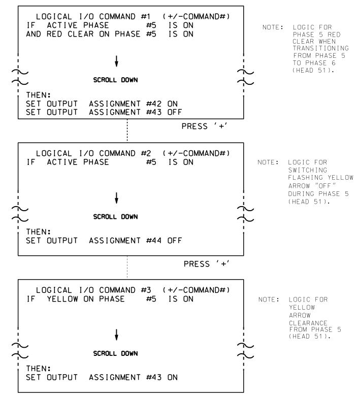
LOGIC I/O PROCESSOR PROGRAMMING COMPLETE
