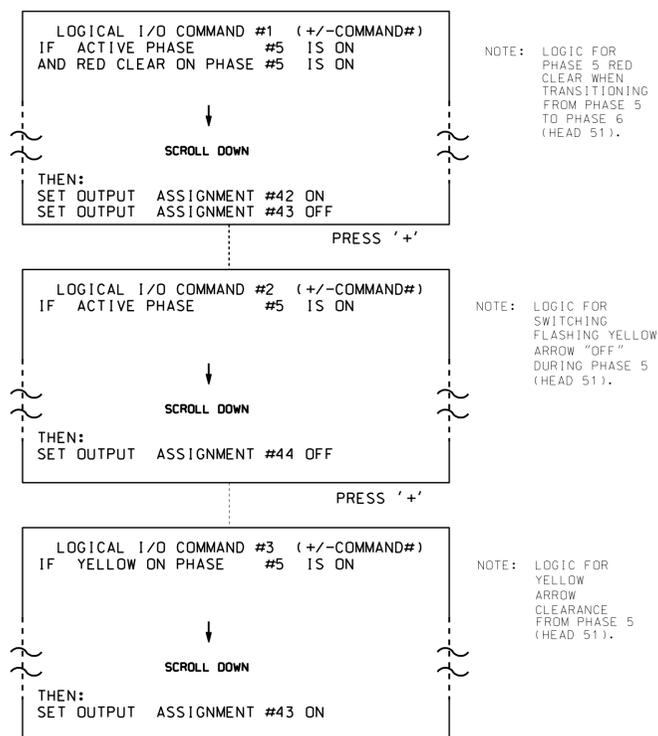
NOTE: LOGIC FOR PHASE 5 RED CLEAR WHEN TRANSITIONING FROM PHASE 5 TO PHASE 6 (HEAD 51).
