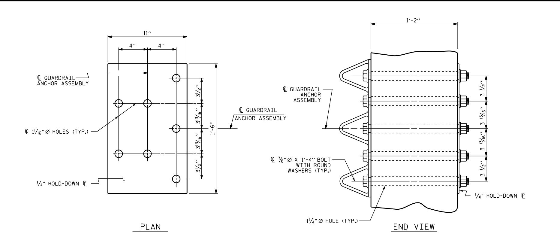
GUARDRAIL ANCHOR ASSEMBLY DETAILS
