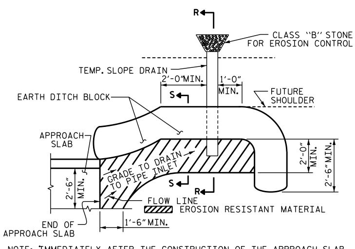
NOTE: IMMEDIATELY AFTER THE CONSTRUCTION OF THE APPROACH SLAB, THE CONTRACTOR SHALL PROVIDE TEMPORARY BERM AND SLOPE DRAIN. CONTRACTOR SHALL GRADE TO PIPE INLET AND PROVIDE EROSION RESISTANT MATERIAL AS SHOWN. THE EROSION RESISTANT MATERIAL SHALL BE EITHER 1) ASPHALT PLANT MIX, TYPE 1 OR TYPE 2, MIN. 2" DEPTH, 2) EROSION CONTROL MAT, OR 3) CONCRETE, AS DIRECTED BY THE ENGINEER. THE SLOPE DRAIN SHALL CONSIST OF A NON-PERFORATED TEMPORARY DRAINAGE PIPE, 12 INCHES IN DIAMETER.
