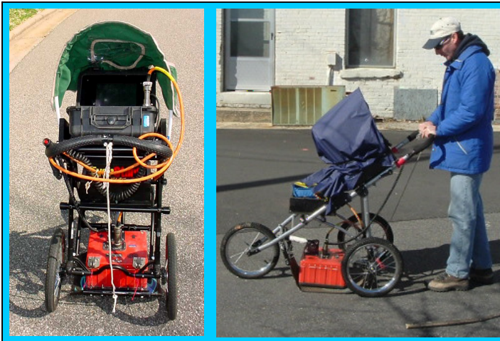
The photographs show the SIR-2000 GPR system equipped with a 400 MHz antenna that were used to conduct the ground penetrating radar investigation across the areas containing steel reinforced concrete and selected EM61 differential anomalies at Parcels, 79, 80, 81, 82, 187, & 188 on August 23 & 29, 2012.
