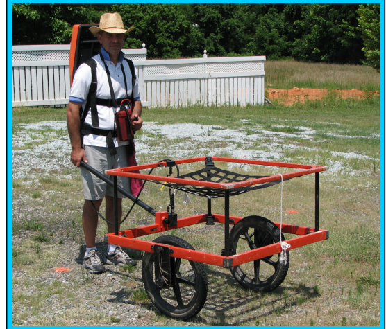
The photograph shows the Geonics EM61 metal detector that was used to conduct the metal detection survey across the Herbert Corey properties (Parcels 79, 81 & 82) on August 22, 2012.
