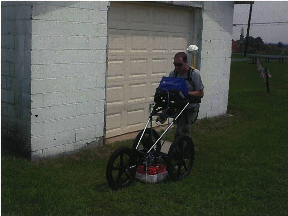
GSSI SIR-3000 Ground-Penetrating Radar with 400 MHz Antenna
