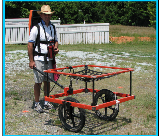
The photograph shows the Geonics EM61 metal detector that was used to conduct the metal detection survey across the Derik A. Sanderson property (Parcel 84) on August 22, 2012.
