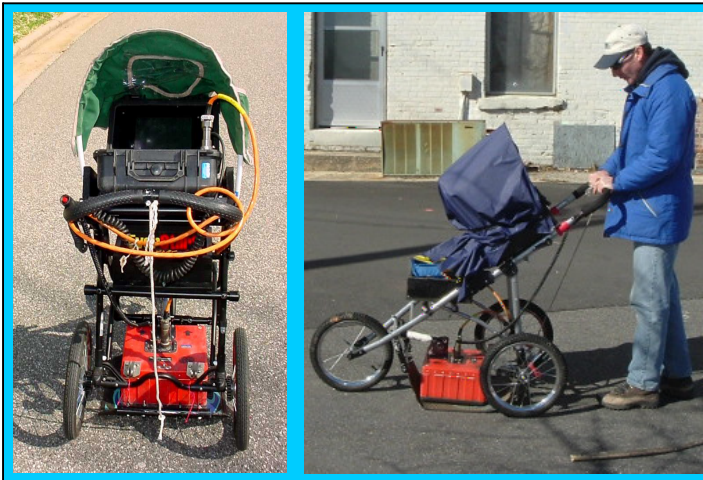
The photographs show the SIR-2000 GPR system equipped with a 400 MHz antenna that were used to conduct the ground penetrating radar investigation across selected EM61 differential anomalies at the Parcel 84 site on August 24, 2012.
