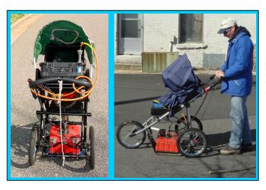
The photographs show the SIR-2000 GPR system equipped with a 400 MHz antenna that were used to conduct the ground penetrating radar investigation across selected EM61 differential anomalies at the Parcel 74 site on August 24, 2012.
